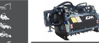
Self-leveling Road Planer with the purpose of dismantling asphalt of the road surface, concrete in squares and scraping the rock or simply creating crossings or tracks on paved surfaces. It is produced in 8 models from 25 to 100 cm wide and can be easily mounted on Skid steer loaders, backhoes and hydrostatic wheel loaders.
